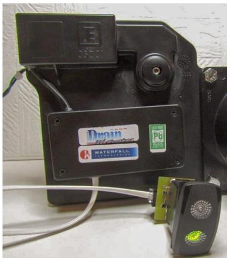
Our Pro-Series valves differ from the Standard and the Premium because they have a computer module on the back. The color and quantity of the wires coming out of the module and connecting to the switch will determine which version you have. This is the original **SVT valve** which has 1 or 2 white RJ11 (phone type) cables coming out of the bottom of the module. It has been discontinued, so please call us to discuss your options.
