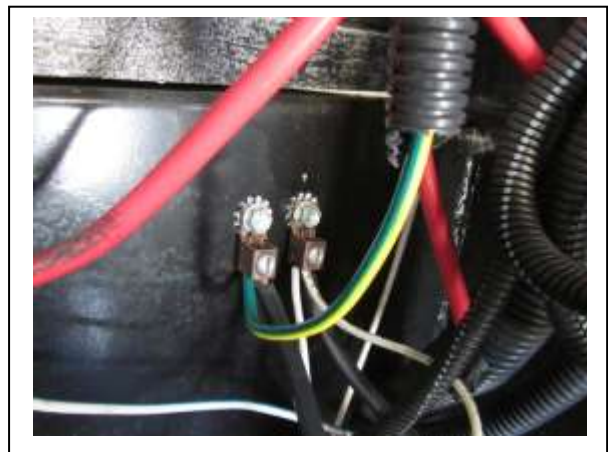
Fig. 16 Tie to Ground lug (-12V) connected to battery -ve terminal
