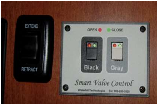
Fig. 18 C Double switch panel mounted (Note: no rear access after panel mounting)
