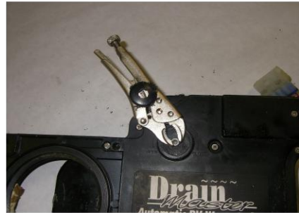
Vice grips on shaft donut removed
