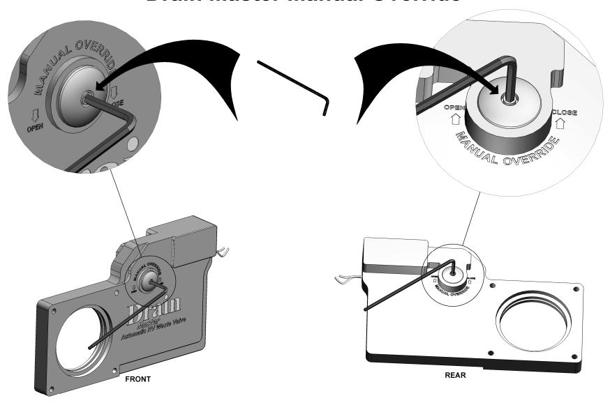
Determine which side of the Drain Master valve you are looking at (label is on the front). With a 1/8" allen wrench, turn the manual override in the appropriate direction (open or close) per the illustration above.
