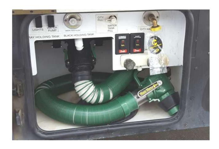
Waste Master 'Always Connected' Hose System installed with in-bay hose storage. Vent Kit seen on female Cam Loc fitting.
