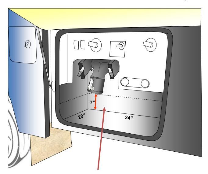
Min. clear space required for WM Hose System install is 24"W x 20"D x 7"H below plumbing terminations. female Cam Loc shown vertical may be installed horizontal in smaller bays to save space.
