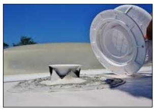
**NOTE:** The funnel channels excess moisture into the holding tank. It protects the roof surface from moisture and helps ensure a tight seal even if the vent pipe is not cut straight.
