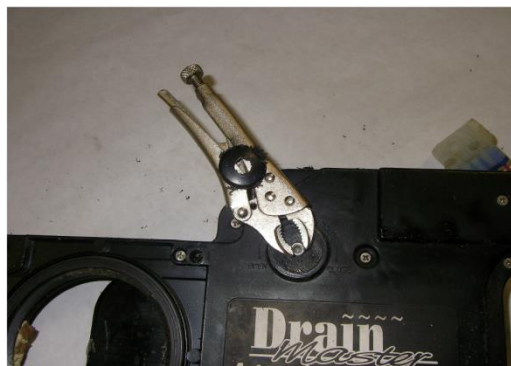
Vice grips on shaft, donut removed
