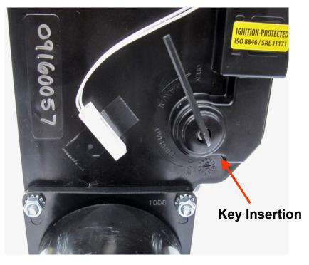
2. Manual override can be performed from either side of the valve – the Front (Label side) or Rear (SN side). Use the side with easiest access. 1 ¼ obstruction free turns of the key will be required. Embossed legends on both sides show: Manual Override, Arrows, Open, Close.
