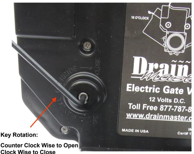
3. With key fully inserted, rotate the key, following the direction arrows:
