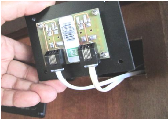
Fig. 17 B RJ 11 ends exit from cutout and plugged into switch panel
